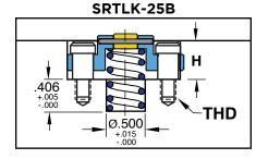
Roller: M M-2 H 60-62 HRC S Titanium Nitride Coated 80 HRC
