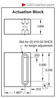
Note: The width of the Actuation Block is smaller by 1/16" to allow for clearance if the CounterView Block is recessed into the mold.
